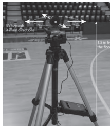
Vertical illuminance (EV) measurement
